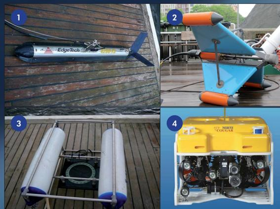
1: Side Scan Sonar EdgeTech 4200; 2: Magnetometer SeaQuest Marine Magnetics; 3: Boomer SIG Energy 3000; 4: SEAEYE COUGAR-XT – a compact, highly flexible and extremely powerful electric ROV with working depths of 2000 meters
