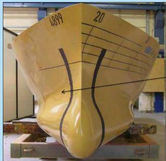
new developed bow with 'dent' to avoid bubble sweep-down
