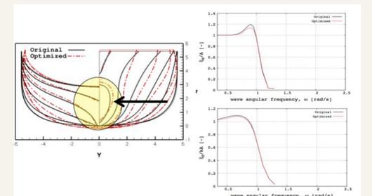
Multi-objective optimization allows for selecting a design on the basis of designer's or ship builder preference: better results in terms of F1 (local flow at the bow), induce a decrease in F2 (seakeeping results).
